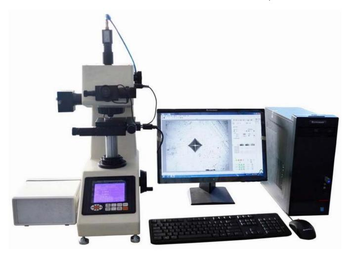
iVick-453MC2 Automatic Micro Vickers Hardness Tester is integrated with several new technologies such as optical imaging, mechanical displacement, electronic control, digital imaging, image analysis, computer processing and so on.
